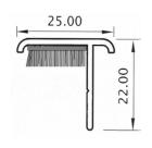
ATB seal incorporates a polypropylene brush seal with aluminium carrier. ideal seal for most internal needs apart from fire, or medium & hot
