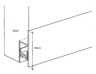
PVC and SILICONE seals both provide an effective barrier to weather, cold smoke, drafts, dust, and noise & smell. Due to its higher temperature melting point silicone is deemed to comply for use as a medium smoke seal for temperatures up to 200°C.
